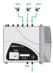
TV multichannel output to the wide band amplifier
